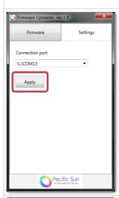
**7.** In the "**Settings**" tab, choose the port COM **number** the device is installed on the computer and click **Apply**
